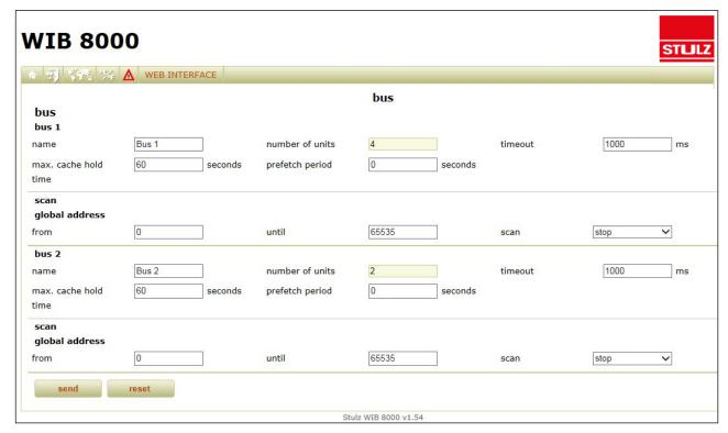
The bus will be configured automatically, when you initiate the WIB module to scan the bus and to record all units found in the bus configuration.
